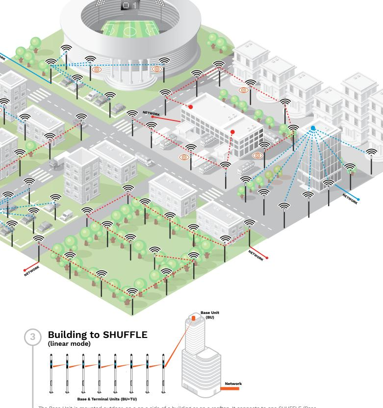
The Base Unit is mounted outdoor, on a on a side of a building or on a rooftop. It connects to one SHUFFLE (Base and Terminal Units) that itself connects to another SHUFFLE having the same hardware (BU+TU) and so on, in a daisy chain layout. The spacing between two SHUFFLEs can reach up to 400 metres (max).
