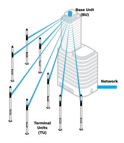
The Base Unit is mounted outdoor, on a side of a building or on a rooftop. It connects to 8 SHUFFLE (Terminal Units) installed within a range of max. 400 metres.
