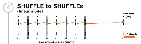
The Base Unit is integrated in a SHUFFLE. It connects to one SHUFFLE (Base and Terminal Units) that itself connects to another SHUFFLE having the same hardware (BU+TU) and so on, in a daisy chain layout. The spacing between two SHUFFLEs can reach up to 400 metres (max).
