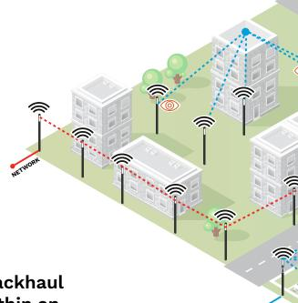
The SHUFFLEs equipped with Wireless backhaul modules communicate in a 90° sector within an unobstructed line-of-sight between radios, with a range of up to 400 metres. Four typical designs are possible.
