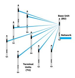
The Base Unit is integrated in a SHUFFLE. This one connects to 8 SHUFFLE (Terminal Units) installed within a range of max. 400 metres..
